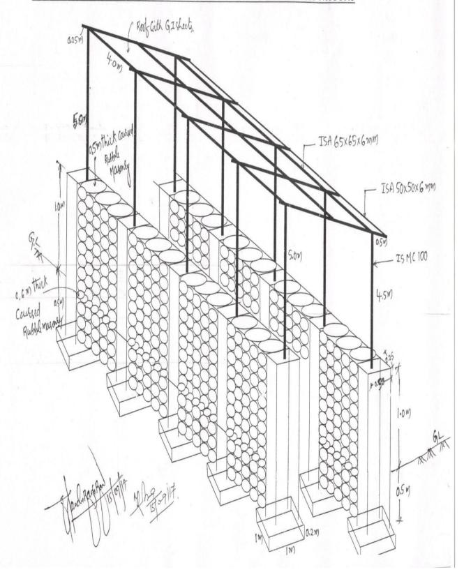
Construction of Platform & shed along the Railway track-for stacking of fly ash bags-for transportation through Railway wagens.
