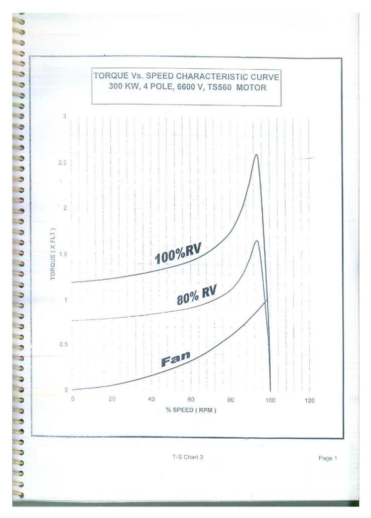
Technical Specification of existing 6.6 KV, 1488 RPM, 3 Phase, 300 KW, Mill Fan Motor.
